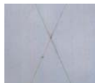
Samsung rust free cabinet material after 1000 hours
