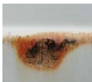
Normal cabinet material after 600 hours
