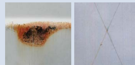
Normal cabinet material after 600 hours
