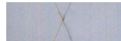
Samsung's rust-free cabinet material after 1000 hours
