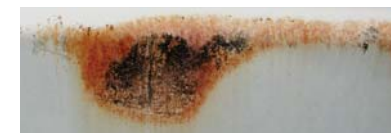
Normal cabinet material after 600 hours
