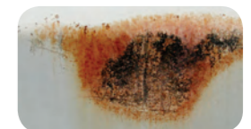
Normal cabinet material after 600 hours
