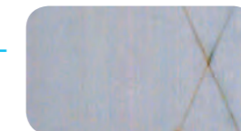
Samsung's rust-free cabinet material after 1000 hours
